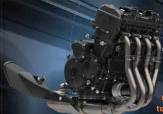
999cm 3 4-stroke, 4-cylinder, liquid-cooled, DOHC engine
